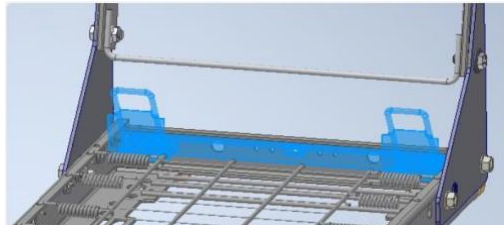
Figure 4-Bracket (blue) in install location.
