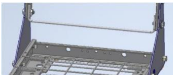
Figure 4-Frame before install showing back-channel location.
