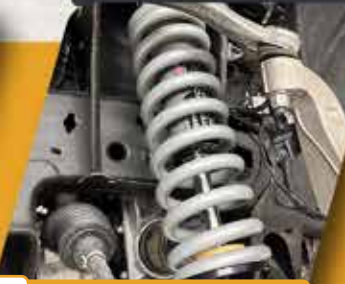
T405 ADS Mesa 2.5" Performance Front Coilovers and Rear Shocks
