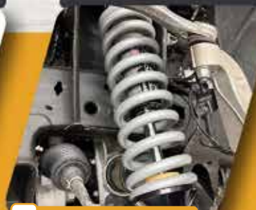
T405 ADS Mesa 2.5" Performance Front Coilovers and Rear Shock
